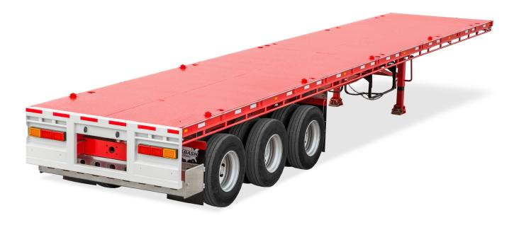
Our rugged steel flatbed trailer is built to last. Heattreated, 900 MPa steel provides high strength and low trailer weight. In addition, the premium paint process ensures best-in-class corrosion resistance and keeps your trailer looking good year after year.
